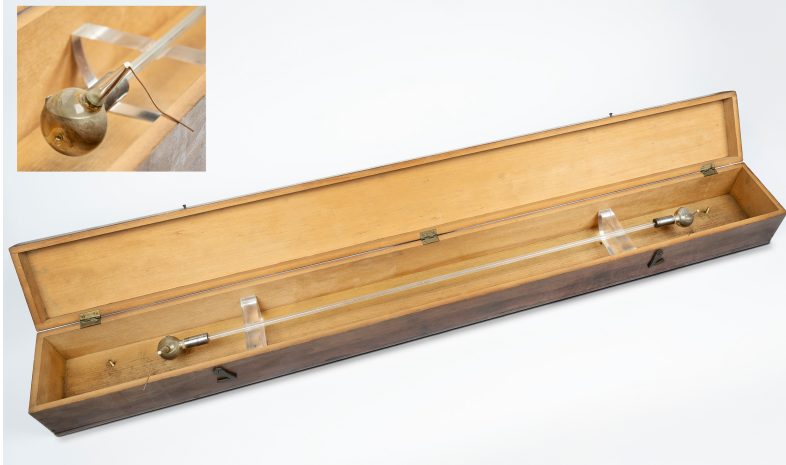
Fig. 2 Mercury ohm according to the 1898 German Imperial Law “Concerning Electrical Units of Measurement”, Implementation Regulation for the International Ohm. Museum display of the Physikalisch-Technische Bundesanstalt, courtesy of H. Scherer.
