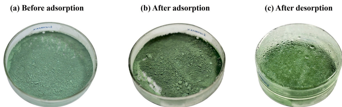
Fig. 10. Visual changes in MIL-101(Cr) during the adsorption–desorption cycle: (a) dried powder before adsorption; (b) after adsorption at 50% RH and 25 °C; (c) after desorption showing condensed water droplets.
