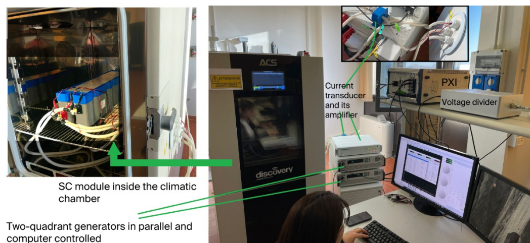
Figure 4. The generation and measurement system for the 130 F module. The current transducer in the image is the LEM IT 205-S Ultrastab for the 80 A peak, which was replaced with a LEM ITZ 2000-50-PR transducer and related amplifier in the case of the 440 A peak.
