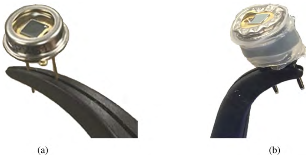
Figure 7. BPX 61 diode (a) unaltered and (b) altered with removed glass cover, flattened casing, and heat shrink tube wrapping. This diode was selected as our detector for its commercial availability and low cost. Alterations to the device were performed to enable low-energy electron detection in a high magnetic field.
