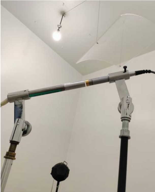
Figure 2. Reference LS2 HBK 4180 microphone (right) faced to the test STEVAL-MKI139V5 MEMS microphone fit into the custom cartridge (left) for pressure-comparison calibration inside the reverberation chamber.
