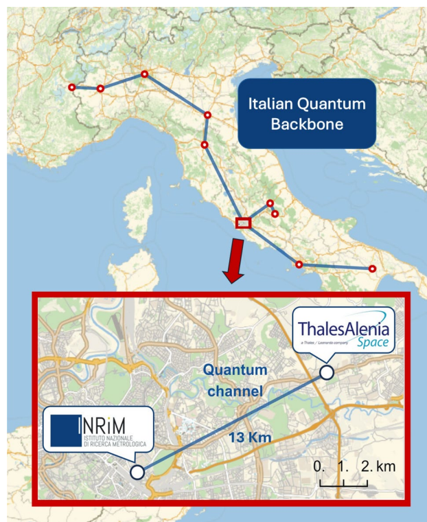
Fig. 1. Schematic representation of the Italian Quantum Backbone showing the main links. The inset shows the fiber link, inside the city of Rome, on which our technique was experimentally carried out. The maps in this figure were generated using the free OpenStreetMap software, released under the Creative Commons Attribution-ShareAlike 2.0 (CC BY-SA 2.0) license.
