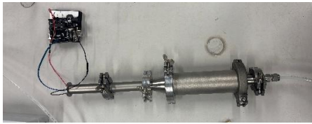
Fig. 3. Linear AISI 304L stainless steel tube with a narrower end into which the low-cost sensor is inserted
