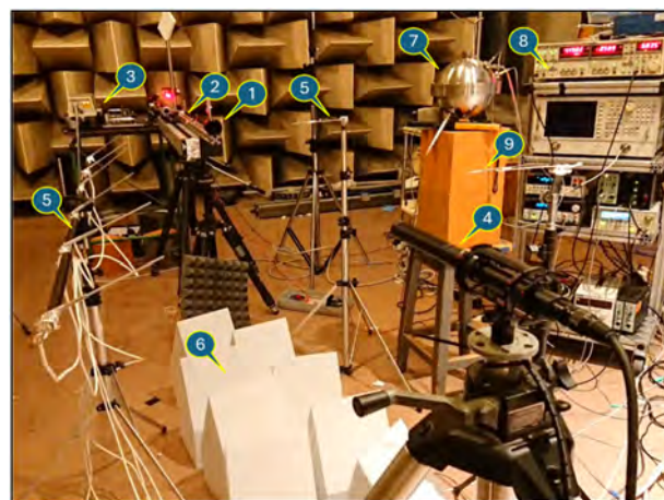
FIG. 10. Experimental setup in a hemi-anechoic chamber for comparison of speed of sound measurements in air with an acoustic wavelength meter and a spherical acoustic resonator. At the background/left is visible the loudspeaker (1) mounted on the moving carriage (2) under the control of an interferometer (3). At the foreground on the right is visible the microphone on the tripod (4). At the left the array of resistance thermometers (5). On the floor foam absorbers for reducing acoustic reflection (6). Top right the spherical resonator (7) with the related electronic bench (8). A hygrometer and a pressure sensor (9), together with a \text{CO}_2 sensor, complete the environmental parameters measurement.
