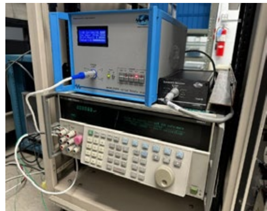
Figure 5. Photo of the measurement setup for artifact calibration of a J. Fluke 5720 MFC (below) with the VRMS (above).
