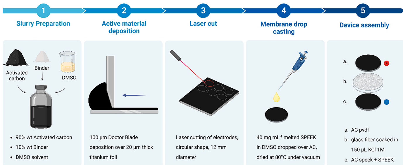
Fig. 2. Flowchart of electrodes and device production process.
