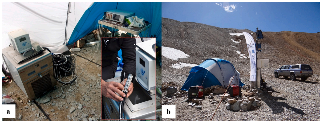
Fig. 2. The mobile calibration facility at Sommeiller Pass during the 2017 campaign. a) Inside the shelter: thermostatic bath and high-accuracy readout bridge, grouped permafrost sensors chain with reference sensors. b) Outside: 100 m permafrost borehole, shelter and power generators.
