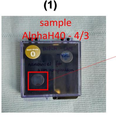
The silicon chip with NWs is installed with carbon tape onto a metallic disk
