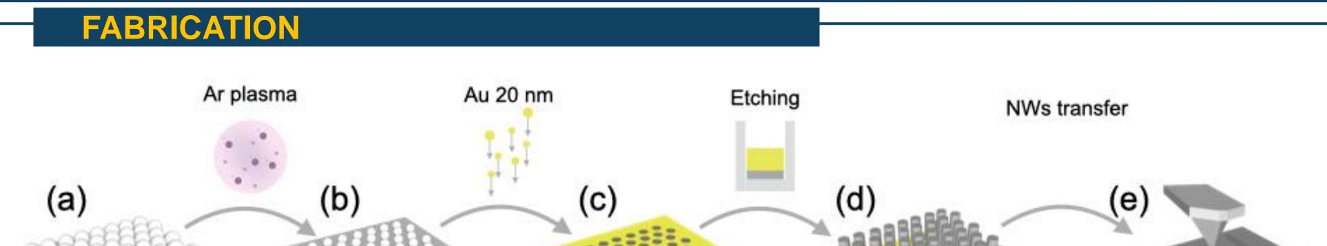
(a) Deposition of polystyrene nanospheres NSs (diameter 200 nm) on the silicon wafer by spin coating at different rotational speed. (b) Reduction of NSs diameter to 100 nm by argon plasma. (c) Deposition of 20 nm of Au and lift-off of the NSs to obtain the pattern of circular voids on the gold layer. (d) Metal-Assisted Chemical Etching to obtain the porous silicon
