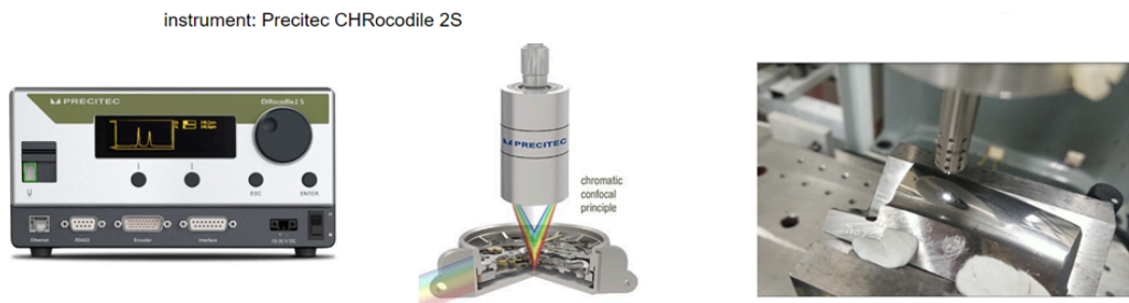
Figure 5: CCPS, Precitec CHRocodile 2S.
