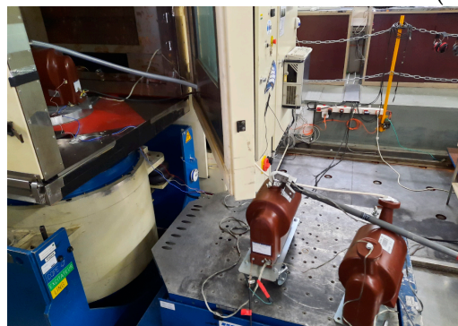
Figure 2. Assessing VT frequency response under temperature and vibration. (a) Scheme of the measuring system; (b) overview of the whole setup arranged at LNE; (c) detail of the generator and the voltage standard transformer, (d) DUT mounted onto the shaker inside the temperature chamber.
