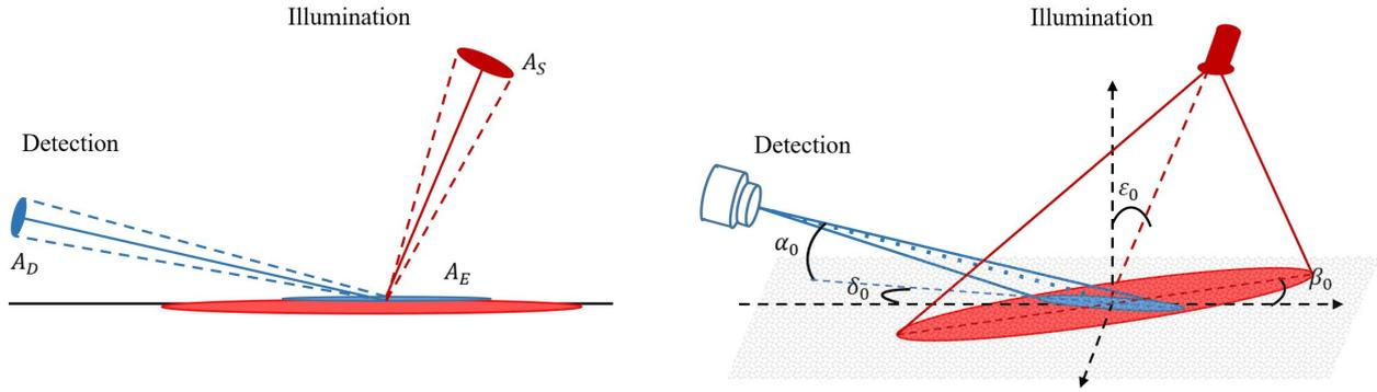
Figure 1. A schematic of the geometrical effects with left) apertures of the illumination  $A_S$  with coordinate system  $(x_S, y_S)$ , of the detection  $A_D$  with coordinate system  $(x_D, y_D)$  and of the effective illuminated area  $A_E$  with coordinate system  $(x_E, y_E)$ ; right) the nominal angles  $(\alpha_0, \delta_0)$  of the detector and  $(\beta_0, \epsilon_0)$  of the source.
