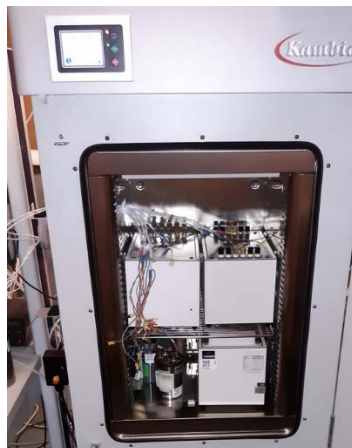
Fig. 3 - 10 k \Omega standards air-bath. The resistors were placed inside a Kambic air-bath mod. 105 with a set-point of 23.000°C and a short-term stability of approximately 0.005°C. The temperature was monitored with a PT100 platinum thermometer.
