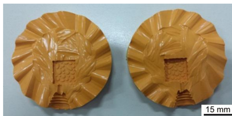
Figure 1. Silicone rubber mold for the metal bezel.
