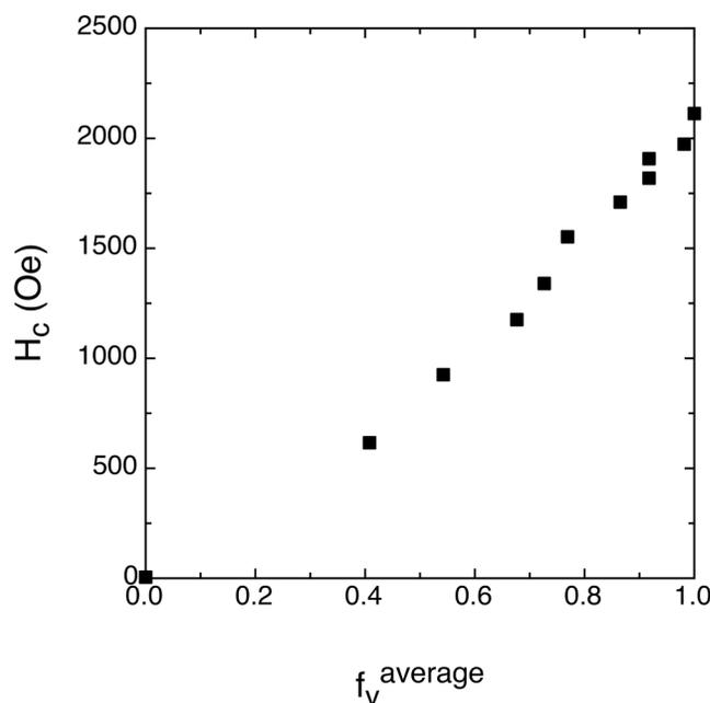
**FIG. 5.** Coercive field as a function of the average transformed volume fraction.
