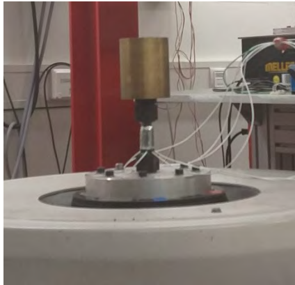
Figure 45 self-manufactured strain gauge on the electrodynamic shaker
