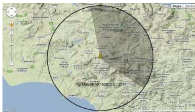
Fig. 3. Map example (no rain) projected over a cartographic system provided by Google©. The image refers to the radar installed in Bisacchino (PA). The gray area is the graphical representation of a blanked region.
