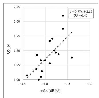
**FIGURE 3** Linear regression graph showing the dependency of the average values across classes of the answers to the question Q5\_N (i.e., "The noise present when you perform a task in silence seems you.") on the slope of the voice signal, mL<sub>S</sub>.
