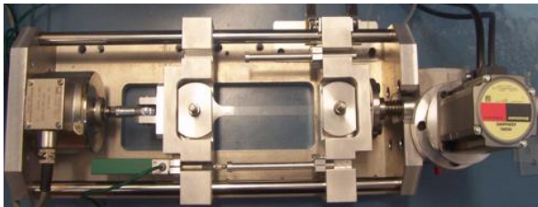
Figure 2: MTM used at INRIM for soft materials
