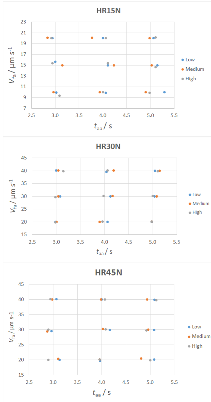
Figure 4: Experimental plans, for the three superficial Rockwell hardness scales HR45N, HR30N and HR15N.
