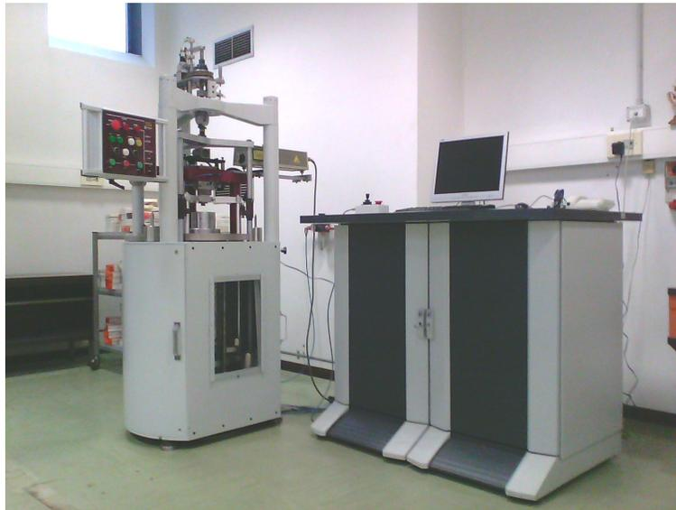
Figure 2: Primary Hardness Standard Machine at INRiM
