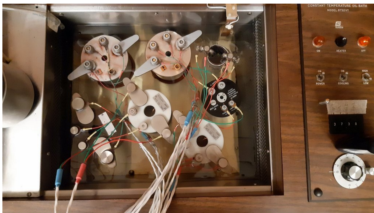
Fig. 2 - Guildline 9732 VT oil bath. The short-term stability of the bath is approximately 0.001°C
