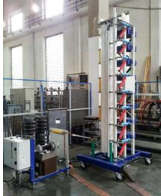
Fig. 2. LATFC's Haefely Impulse generator.
