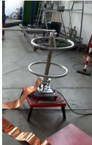
Fig. 1. SAGI 304 resistive divider up to 200 kV.
