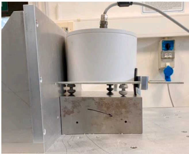
Fig. 5. The seismometer on the inclined plane ( 2^\circ \pm 0.1^\circ ).
