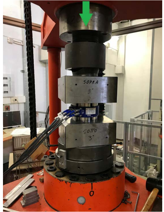
Figure 4. The 1 MN deadweight FSM integrated with 3° tilted plates at INRiM.
