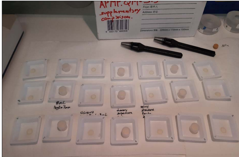
Figure 5: The 9 cylindrical tablet samples in their cut 3 mL PE irradiation vials and the 12 As standard discs.
