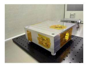
Figure 2: real picture of machined aluminum chamber
