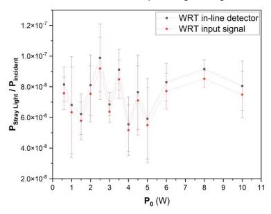
Figure 8: plot showing how the stray photons change their power as the power of the light source varies in the range  $(0.6 \div 10)$  W; each point averages the results of three consecutive simulations
