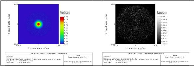
Figure 6: irradiance plot of the spot visualized on the in-line detector (on the left) and stray light signal in the "reference" condition of no iris diaphragms and no coatings and absorbers installed inside the chamber
