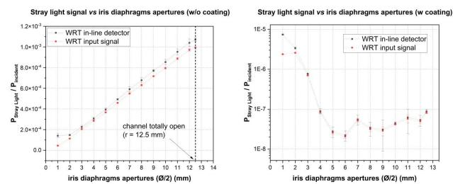
Figure 7: plots of the irradiance ratios of the signals with respect to the apertures of the iris diaphragms, without (on the left) and with 99.5 % absorbance coating applied (on the right)
