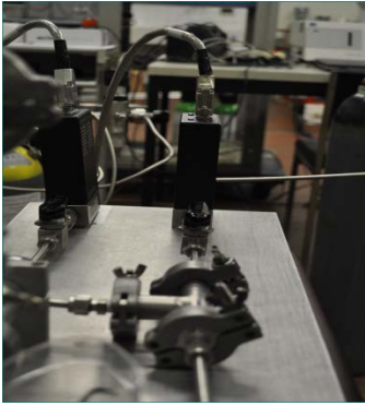
Fig. 3: Dynamic dilution system composed by two Mass Flow Controllers and a mixing chamber.
