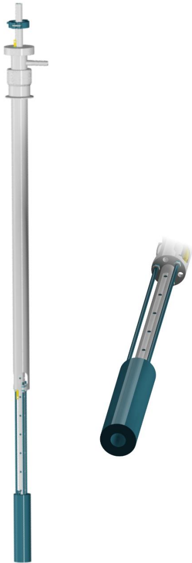
Figure 1. A computer rendering of the cryomagnetic probe assembly: (left) side view; (right) front view, showing the magnet bore.
