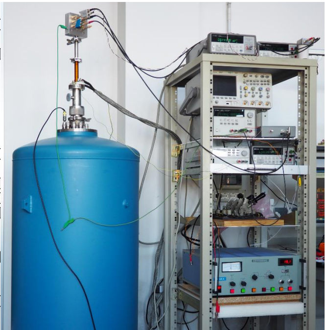
Figure 7. Overall view of the measurement setup for DC characterization. On the left, the liquid helium dewar, with the coaxial probe inserted. On the right, the rack of electronic instrumentation.
