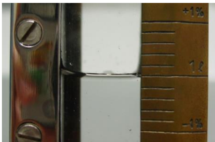
Figure 1. Standard test measure meniscus
