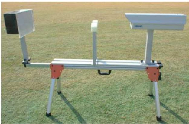
**FIGURE 7** Image of the high-speed optical disdrometer
