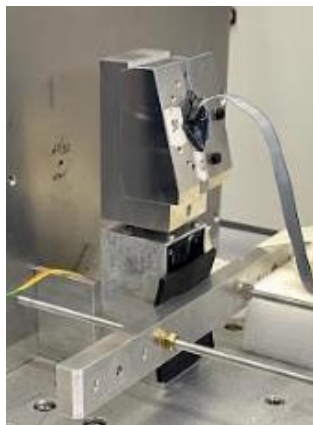
Figure 10. The experimental set-up with the stepper motor on the horizontal vibrating table.
