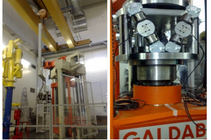
Figure 3. The HS MCFMT during the first calibration in the 1 MN deadweight FSM at INRiM.
