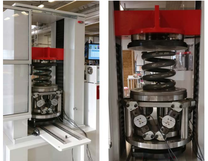
Figure 4. The first multicomponent spring testing machine by Easydur Italiana during spring tests.
