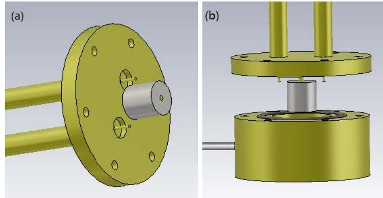
**Figure 1.** a) Top cap of the cavity with the cylindrical sapphire and two antennae probes; b) full opened cavity with O-rings seal, bottom cap with drilled hole, the vacuum line and top cap shown in (a)
