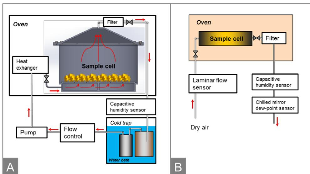
Figure 1: Schematic drawings of the primary standards for water mass fraction developed at a) VTT MIKES and b) DTI. The balances used for weighing the sample cells are not shown in the drawings.
