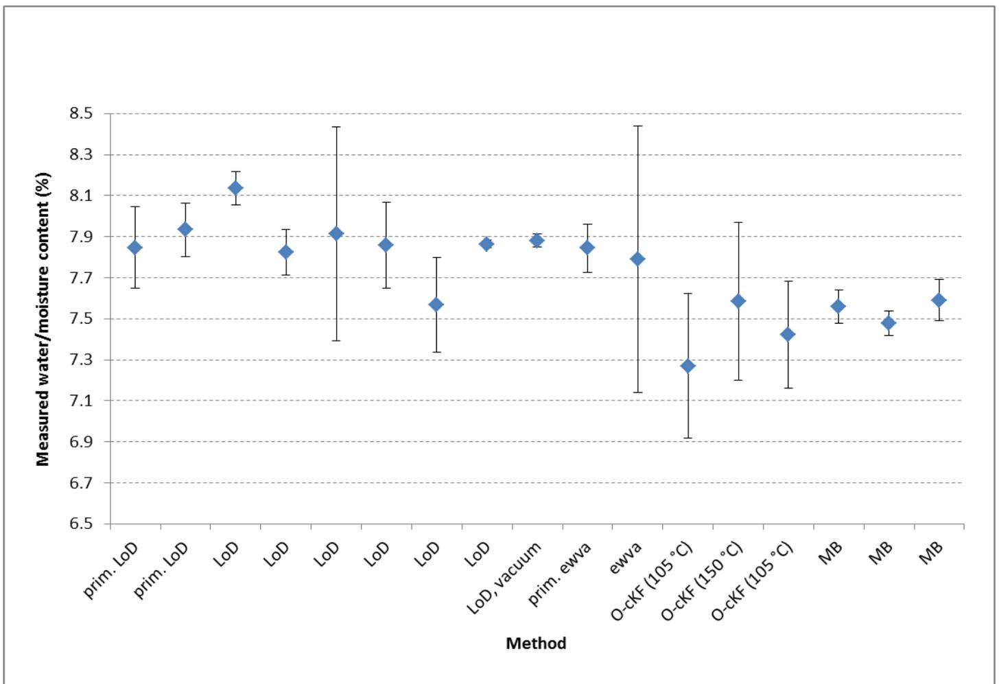
Figure 6: Results obtained with different methods and instruments in the inter-laboratory comparison with wood pellets. O-cKF = coulometric Karl Fischer titrator with oven, ewva = evolved water vapour analyser, LoD = oven drying system, MB = moisture balance. The primary standards are indentified with 'prim'. Error bars show estimated uncertainties at about 95 % confidence level.
