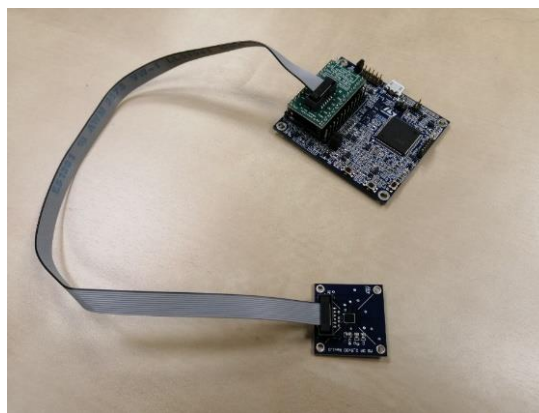
Figure 1. The MEMS accelerometer connected to the IC board.
