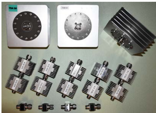
Fig. 4. Set of coaxial shunts built at INRIM and employed for primary alternating current scale realization and as phase standard for currents from 20 mA up to 7 A and frequencies up to 100 kHz.
