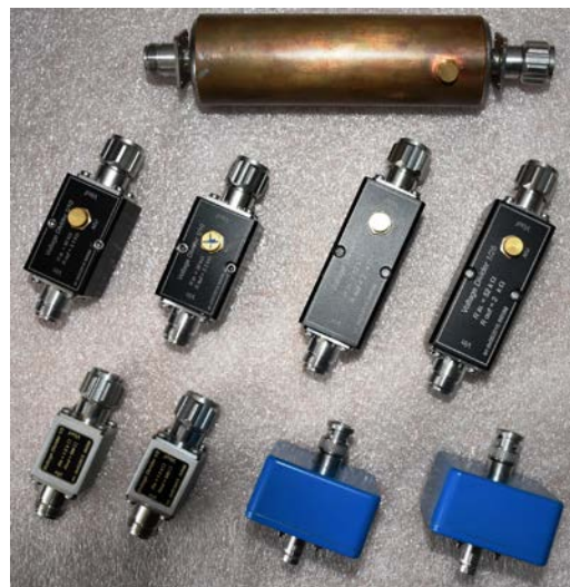
Fig. 3. New set of wideband coaxial resistive dividers for voltages ranging from 1 V to 150 V and frequencies up to 1 MHz. Construction details of 1:52 ratio RVD are given in [7].
