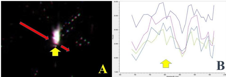
**Fig. 3.** a) Color reconstruction of the hyperspectral image of the welding plasma and well. The arrow highlights the pixels whose spectra are plotted in b) while the overall spectrum acquired through the spectroradiometer is shown in Fig. 2
