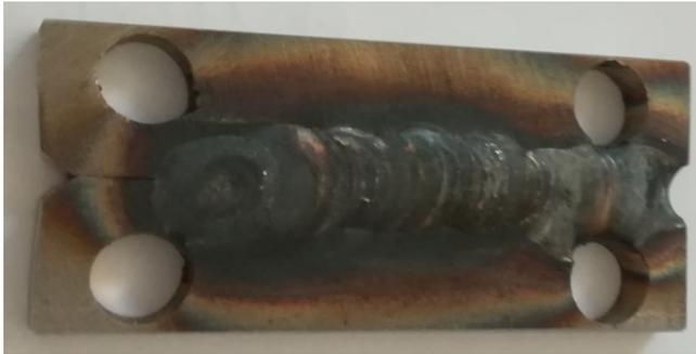
**Fig.4.** AISI sample welded by TIG
