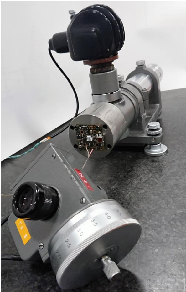
Fig. 1 Picture of the modified Hilger & Watts autocollimator. In the foreground, the old detection system is visible. Behind it, there is the electric circuit of the IDS camera mounted on a steel cylinder used to keep it at the focal plane of the optical system. On top of the picture, the black knurled part is the shield of the lamp. The lamp is powered with a 4V DC source.
