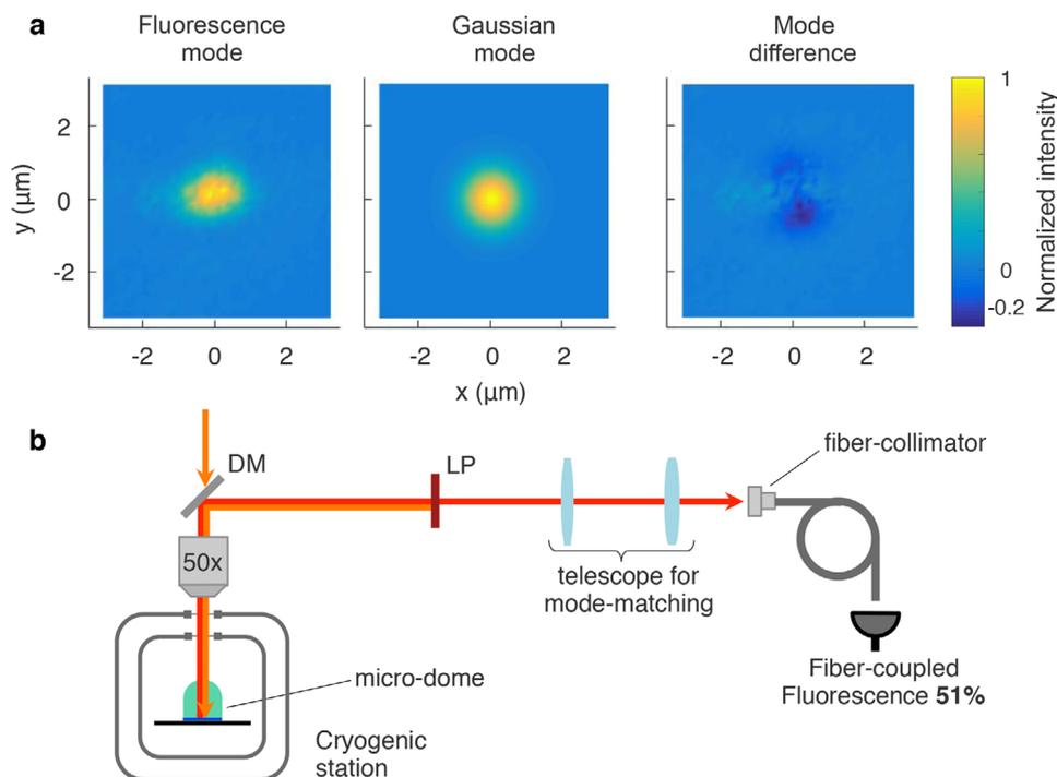
**Figure 5.** Efficient coupling into a fiber. a) The measured fluorescence spatial distribution of the integrated structure is compared to a Gaussian mode, typical of a single mode optical fiber, and the difference between the two profiles is shown on the right. b) Schematic of the fiber-coupling setup, which consists in the objective, a telescope and a tunable-distance fiber-collimator (DM and LP label the dichroic mirror and the long-pass filter respectively—see Experimental Section).
