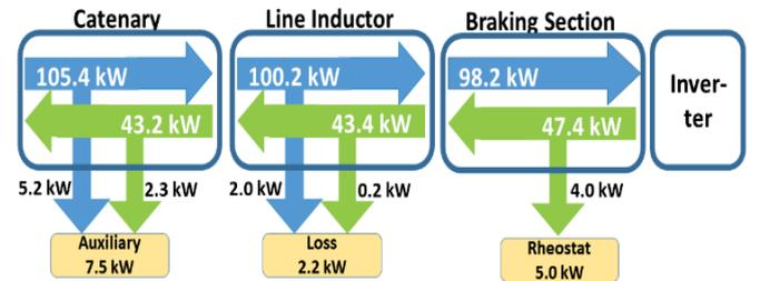
Fig. 7. Average power flows on single traction unit.
