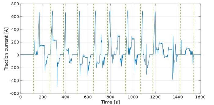
Fig. 5. Traction current ( $I_t$ ) during a one-way trip.
