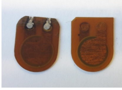
Figure 4. Wide-band ceramic PZT “DuraAct” kapton encapsulated.
