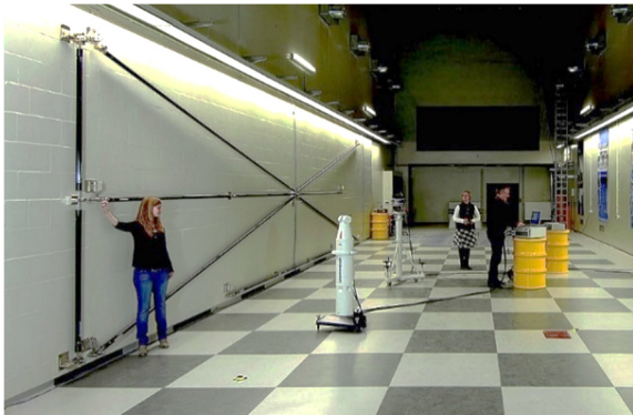
Figure 29. PTB's reference wall for testing and calibrating mobile 3D measuring systems for large measuring ranges up to 12 m (source: PTB).
