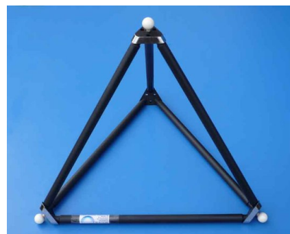
Figure 44. Ball tetrahedron artefact (source: Trapet Precision Engineering).
