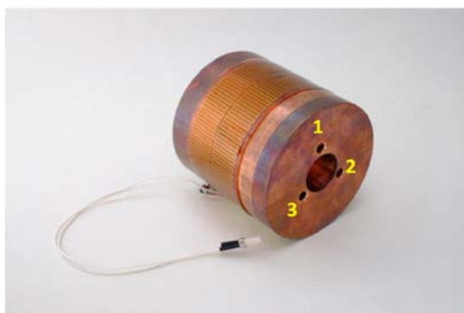
Figure 2: copper cylinder with electrical heater wrapped around it, and the thermometer wells labeled (Figure in color only online)
