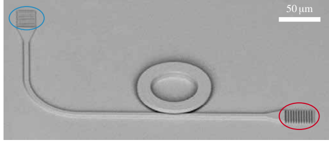
(a) polymer waveguide coupled to a ring resonator (SEM picture)
