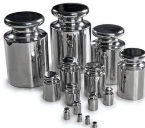
Figure 1: Some weights to be calibrated against limited number of mass standards
