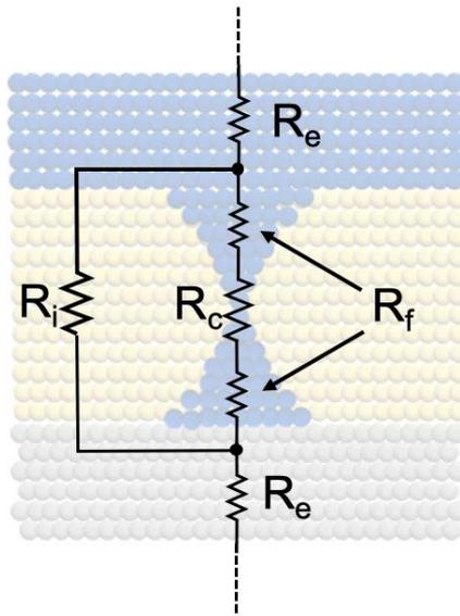
**Figure 5.** Equivalent electrical circuit of a memristive cell. Besides the quantized contact resistance  $R_c$ , the equivalent circuit is composed of the bulk filament resistance  $R_f$ , the resistance of the insulating active materials  $R_i$  and the resistance of the metallic electrodes  $R_e$ .
