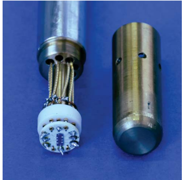
Fig. 3. The bottom side of the insert, which slides into the cryomagnet bore. The brass shield (right) has been removed, to show the TO-8 socket, which hosts a GaAs device on its TO-8 holder, and the 9 coaxial electrical lines.
